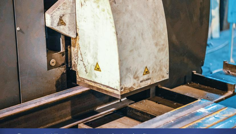
The automatic drilling line speeds up the perforation of profiles.
