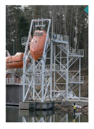
The Ojamo training station's lifeboat rigging can be tilted in both directions. The realism of the training is enhanced by the flow generated by the current machinery.
