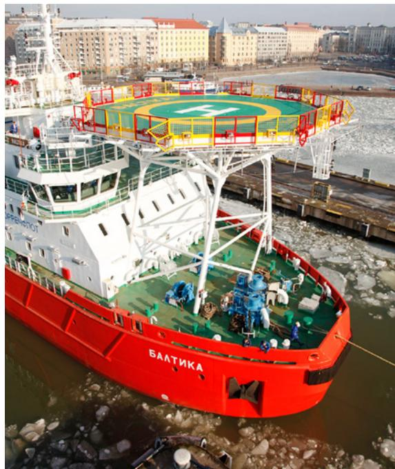
Classification Russian Maritime Register of Shipping: KM ⚙ Icebreaker6, [1], AUT1-ICS, OMBO, FF3WS, EPP, DYNPOS-1, ECO-S, Oil recovery ship (>60°C), Salvage ship, Tug, Helideck
